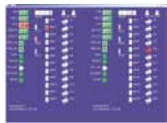
When a fault is detected a PC-connected system logs the fault. The system can also automatically e-mail a user or selected support group the instant a fault occurs. This group could include Federal Signal's Integrated Systems service department, which is able to provide remote support via the internet.
